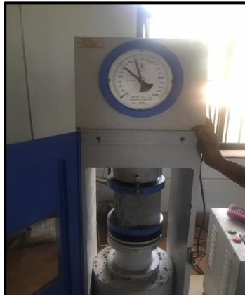
Fig 5: Compression test on cube specimen
