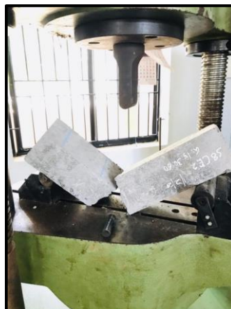
Fig 9: Flexural strength test on beam specimen
