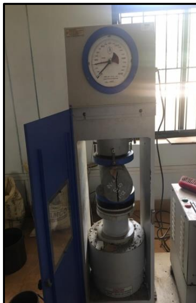
Fig 7: Split tensile test on cylindrical specimen
